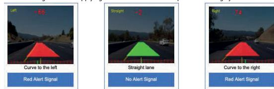
Fig. 3. After applying the model for the lane departure warning system
