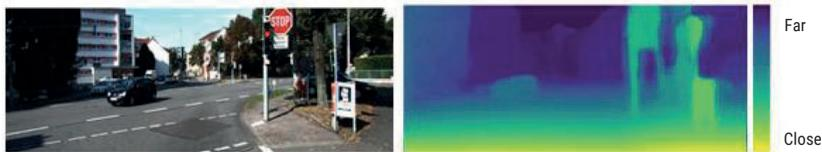
Fig.4. Depth prediction result on KITTI 2015. At left, single view input image. At right, the obtained result of depth map prediction.
