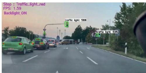
Figure 6: Traffic Light and Backlight Detection
