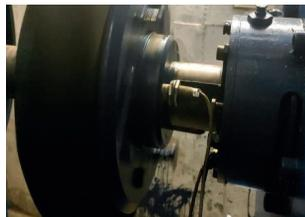
Induction sensor for RPM measuring
