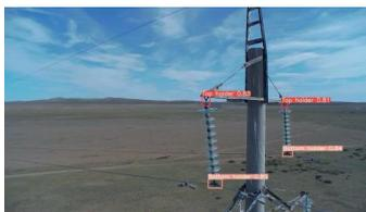
Fig 7 shows a deep learning model for detecting insulator based on YOLOv4.
